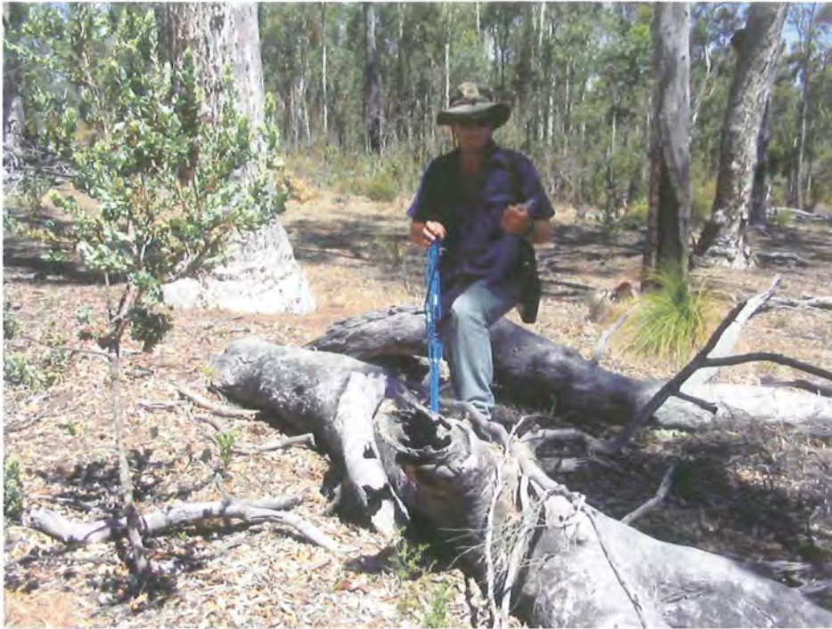
Plate 3.8: Hand-held receiver and antenna used to locate radio-collared specimens and their diurnal refuge sites during the Pro bait trial.
